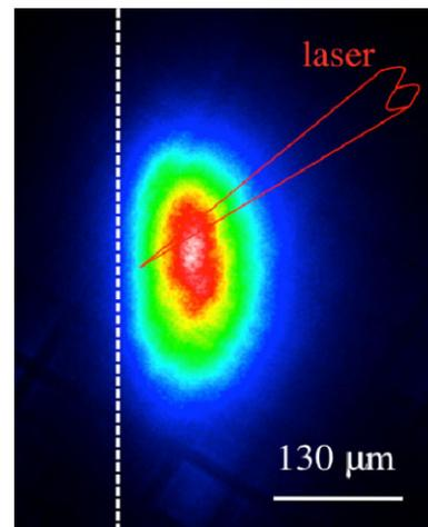
**Fig. 4** In-band EUV image of Sn plasma irradiated with CO<sub>2</sub> laser pulse incident at an angle of 45 degrees respect to the target normal
