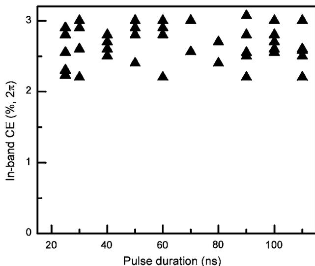
FIG. 2. In-band CE from CO<sub>2</sub> laser-produced Sn plasma as a function of laser pulse duration.
