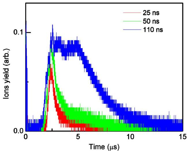
FIG. 4. (Color online) Time of flight of Sn ions from Sn plasma irradiated by CO<sub>2</sub> laser with various pulse durations of 25 (red), 50 (green), and 110 ns (blue).
