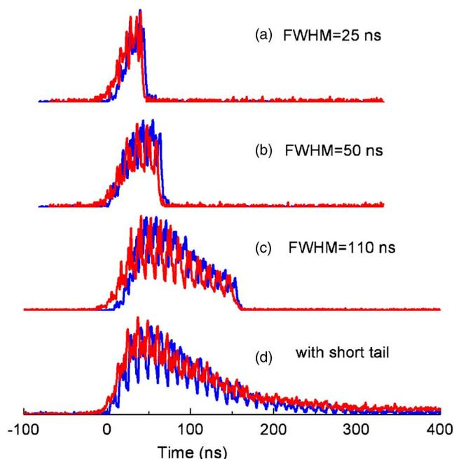
FIG. 1. (Color online) Temporal shape of laser pulse (red lines) and in-band EUV light (blue lines) from Sn plasma irradiated by CO<sub>2</sub> laser with pulse durations of (a) 25, (b) 50, (c) 110, and (d) 110 ns with a short tail.
