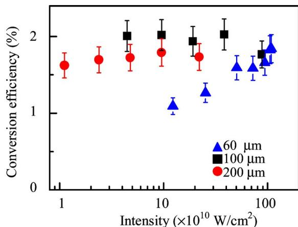
Fig. 1. (Color online) In-band conversion efficiency of laser-produced Sn plasmas using focal spot sizes of 60 (triangles), 100 (rectangles), and  $200\ \mu\text{m}$  (solid dots) versus laser intensity.
