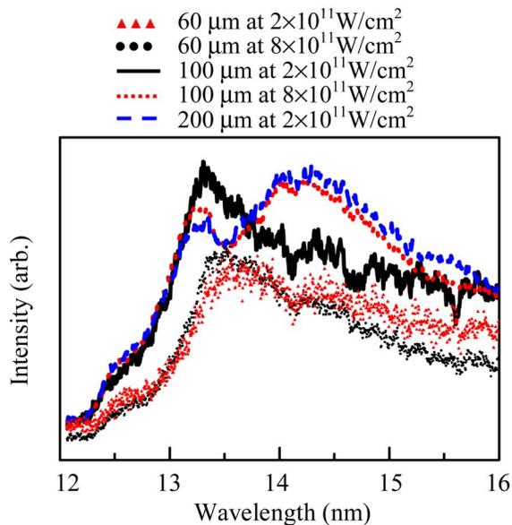
Fig. 3. (Color online) Spectra of laser-produced Sn plasmas using focal spot sizes of  $60\ \mu\text{m}$  at intensities of  $2 \times 10^{11}$  (red triangles) and  $8 \times 10^{11}$   $\text{W}/\text{cm}^2$  (black dots),  $100\ \mu\text{m}$  at intensities of  $2 \times 10^{11}$  (black solid curve) and  $8 \times 10^{11}$   $\text{W}/\text{cm}^2$  (red short-dashed curve), and  $200\ \mu\text{m}$  at intensity of  $2 \times 10^{11}$   $\text{W}/\text{cm}^2$  (blue dashed curve).
