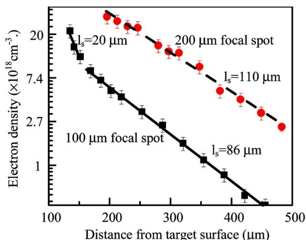
Fig. 2. (Color online) Density profiles of laser-produced Sn plasmas with focal spot sizes of  $100\ \mu\text{m}$  (circles) and  $200\ \mu\text{m}$  (squares) obtained at  $2 \times 10^{11}\ \text{W}/\text{cm}^2$ . The two solid curves represent the exponential decay fit of  $100\ \mu\text{m}$  spot data with scale lengths of 20 and  $86\ \mu\text{m}$ , and the dashed line represents the fit of  $200\ \mu\text{m}$  spot data with a scale length of  $110\ \mu\text{m}$ .
