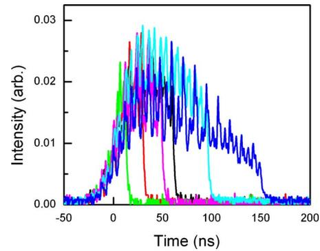
FIG. 6. (Color online) Waveforms of CO<sub>2</sub> laser pulse with various pulse durations cut with the externally triggered plasma switch.
