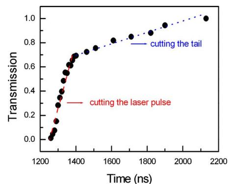
FIG. 7. (Color online) Transmission of air breakdown plasma induced by CO<sub>2</sub> laser as a function of delay times.
