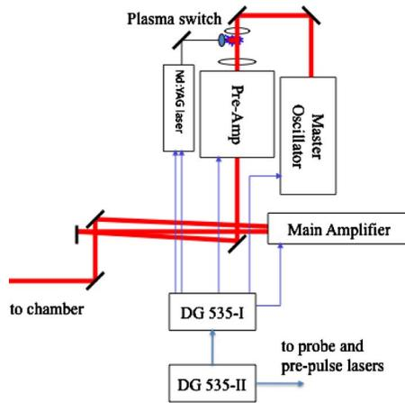
FIG. 1. (Color online) Schematic illustration of the CO<sub>2</sub> MOPA laser system.
