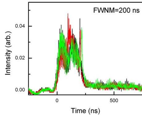
FIG. 2. (Color online) Waveform of CO<sub>2</sub> laser pulse with pulse duration of 200 ns (three shots).
