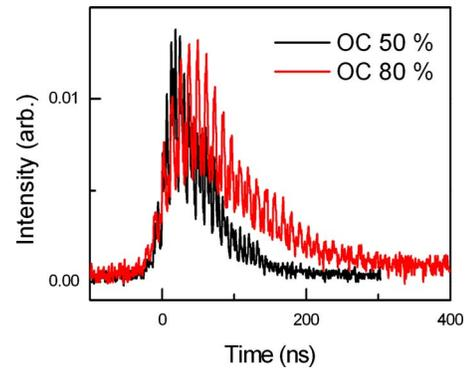
FIG. 4. (Color online) Waveforms of CO<sub>2</sub> laser pulse with output coupler with reflectivity of 50% (narrower one) and 80% (broader one).
