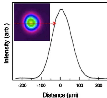
FIG. 9. (Color online) The photo of the focal spot of the CO<sub>2</sub> laser with a 7.5 in. and its intensity profile.
