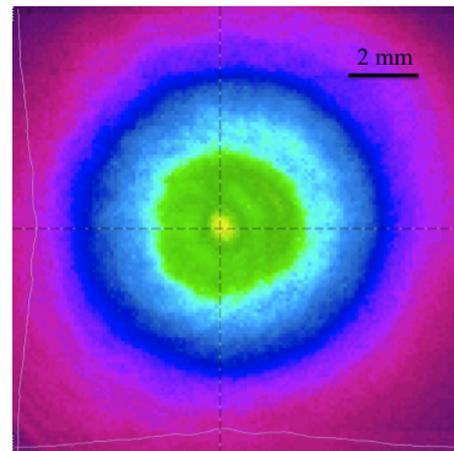
FIG. 8. (Color online) Near field beam pattern of the CO<sub>2</sub> laser.
