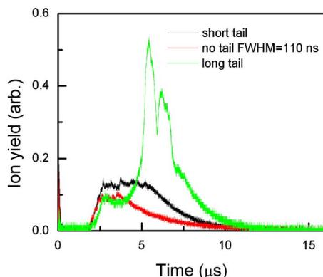
FIG. 10. (Color online) TOF of the ions from Sn target irradiated with a CO<sub>2</sub> laser pulse with long tail (with highest magnitude of flow ions), short tail (with middle magnitude of slow ions), and no tail (with lowest magnitude of slow ions).
