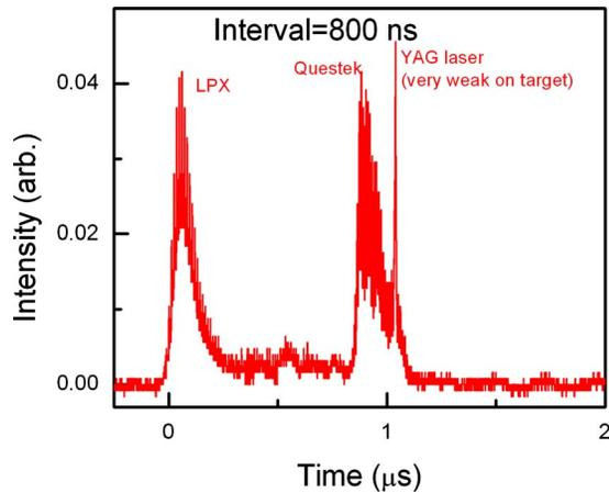
FIG. 3. (Color online) A train of CO<sub>2</sub> laser pulses with an interval of 0.8 μs.
