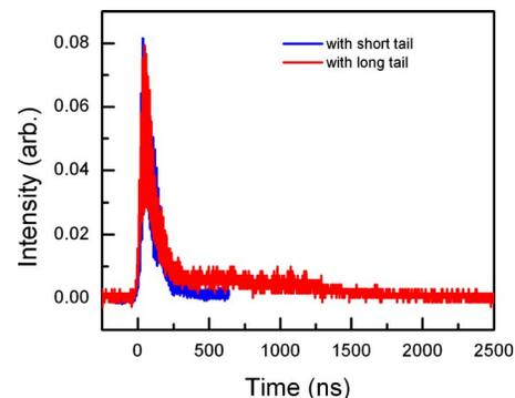
FIG. 5. (Color online) Waveforms of CO<sub>2</sub> laser pulse with gas ratios of CO<sub>2</sub>:N<sub>2</sub>:He=8:10:82% (the one with longer tail) and CO<sub>2</sub>:N<sub>2</sub>:He=20:4:76%.
