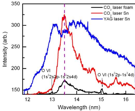
Fig. 3. (Color on line) Soft X-ray spectra from pure Sn target irradiated with (blue line) 1.06 and (red line) 10.6  $\mu\text{m}$  lasers, and from (black line) foam target with 1% concentration of Sn.
