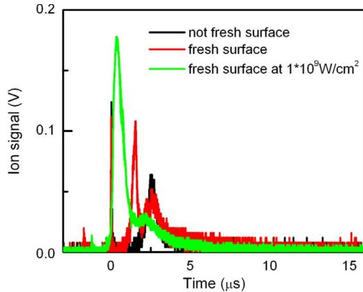
Fig. 2. (Color on line) Time of flights from Sn plate with (red line) fresh surface and (black line) exposed surface irradiated with a CO<sub>2</sub> laser pulse with a laser intensity of  $1 \times 10^{10}$  W/cm<sup>2</sup>, and (green line) fresh target surface irradiated with a CO<sub>2</sub> laser with laser intensity of  $1 \times 10^9$  W/cm<sup>2</sup>.
