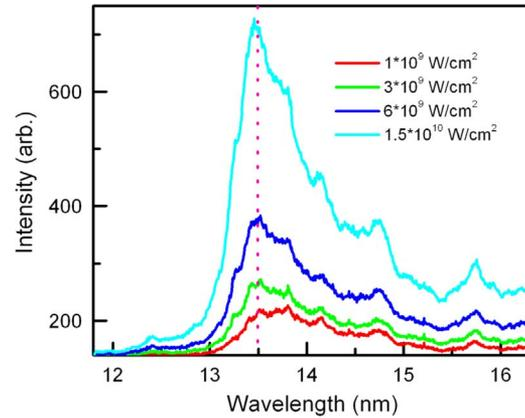
Fig. 1. (Color on line) Soft X-ray spectra from Sn plasma irradiated by CO<sub>2</sub> laser pulses with various laser intensities.
