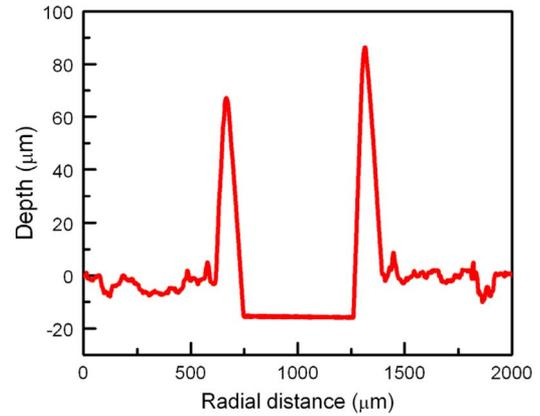
Fig. 5. (Color on line) Profile of the target surface after accumulating 20 laser shots.
