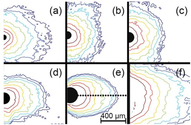
FIG. 3. (Color online)  $\log_{10}$  of the plasma density at the peak of the laser pulse for SD/FSS ratios of (a) 1.11, (b) 1.66, (c) 2.30, (d) 2.48, (e) 3.34, and (f) planar. The contour lines correspond to  $\log_{10}$  values of 17.5–19 in 0.25 increments.
