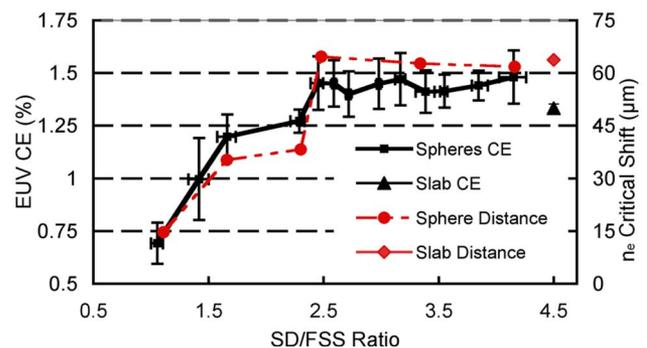
FIG. 1. (Color online) The in-band EUV CE in a  $2\pi$  sr for spheres of 80–330  $\mu\text{m}$  corresponding to a 1.1–4.3 SD/FSS ratio (black squares) and the critical density plasma shift along the laser axis (red circle). Also plotted is the planar target CE (black triangle) and critical density shift (red diamond).
