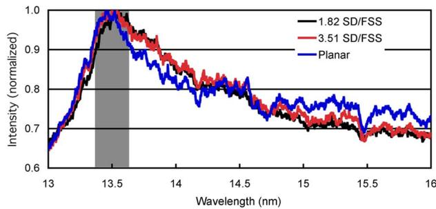
FIG. 5. (Color online) Typical soft x-ray spectra at  $45^\circ$  for SD/FSS ratios of 1.82, 3.51, and planar with the in-band EUV region shaded.
