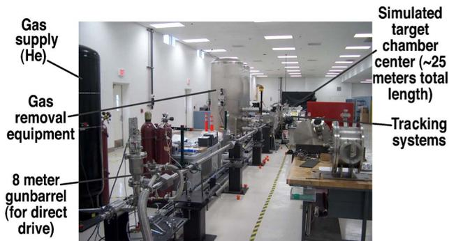
FIG. 4. Injection demonstration to simulate the full-length of a laser IFE fueling system, based on the Sombrero laser fusion power plant.
