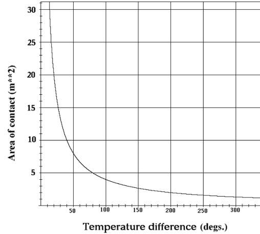
Fig. 4 Area required to remove 2 MW of power vs. temperature difference, assuming contact conductance =  $5000 \text{ W/m}^2$ .
