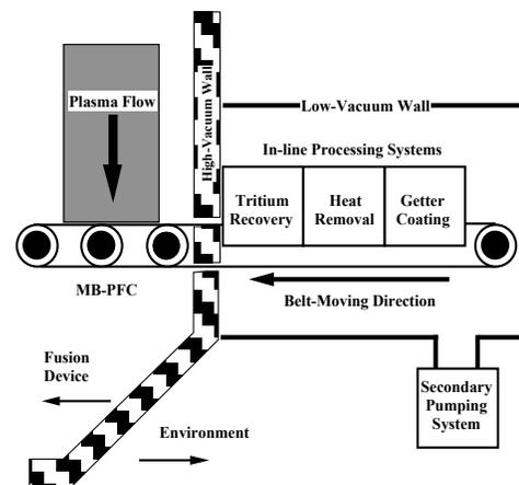
Fig. 1 The moving-belt PFC concept with ex-situ inline belt processing systems for tritium recovery, heat removal and getter coatings.
