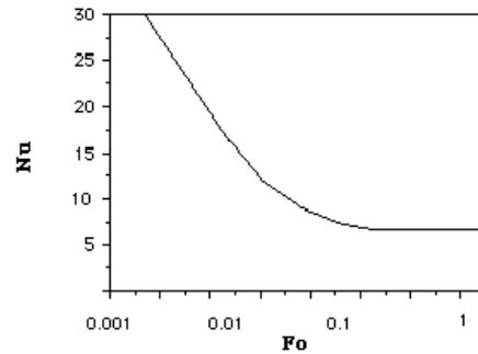
Fig. 5 Heat transfer coefficient expressed by the Nusselt number vs. Fourier number.
