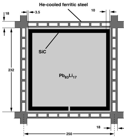
Fig. III. Configuration of a breeding zone cell.
