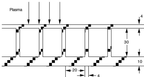
Fig. II. Cross section of the first wall box
