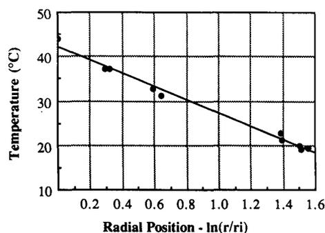
Figure 4. Typical radial temperature distribution, including temperature jump at the wall (4.3 mm Al + 1 atm He)
