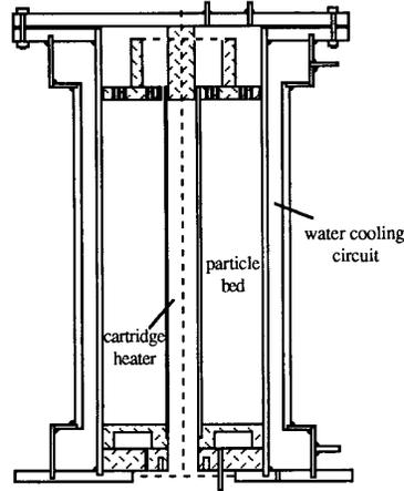
Figure 3. Diagram of test section
