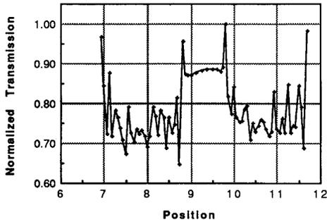
Figure 1. Porosity profile for a single-size bed
